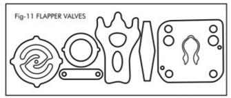
stressed precision spring steel components requires resistance to flexing fatigue, high impact loads and extreme operational stresses. To meet the demand of surface refinement and controlled redious on difficult inside edges. For certain compressor and two-cycle applications which requires the highest degree of precision and dependability, shot peening is recommended.
