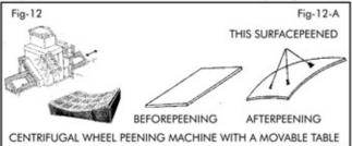
abrupt changes in contour. It is best suited for forming curvatures where the redious are within the metal's elastic range. The sketch below shows an integrally stiffened wingskin being peened in peen forming machine, which has the necessary controls to achieve varying curvature requirements along the skin while compensating for varying thickness, cutouts and reinforcements, as well as distortion caused by machining or heat treatment.
