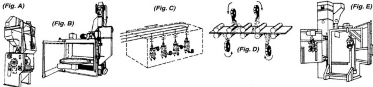
**Roller & Belt Conveyor Machine (Fig. D) :** This picture shows plate, sheet or structural shape descaling at high speed. Both upper and lower surfaces are shot blasted simultaneously.
